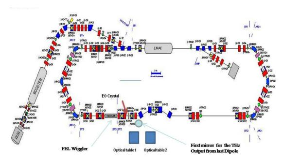
Figure 1: The EO experiment is located on the optical tables shown. The probe beam is injected through the bend in the last dipole magnet and then goes through the EO crystal and then arrives at the optical table 1 for decoding. The Coherent Synchrotron Radiation (CSR) THz output port is located near optical table 2 so that implementing the measurement is achieved with the same setup. This also shows the position of the Wiggler for the FEL.
