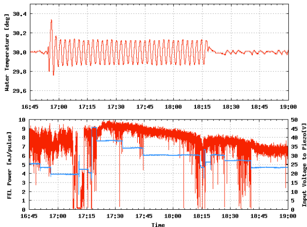
Figure 4: Time variation of the temperature of the fine cooling water (upper), the optical power of FEL (lower, red) and the adjusted input voltage to the piezo actuator (lower, blue).
