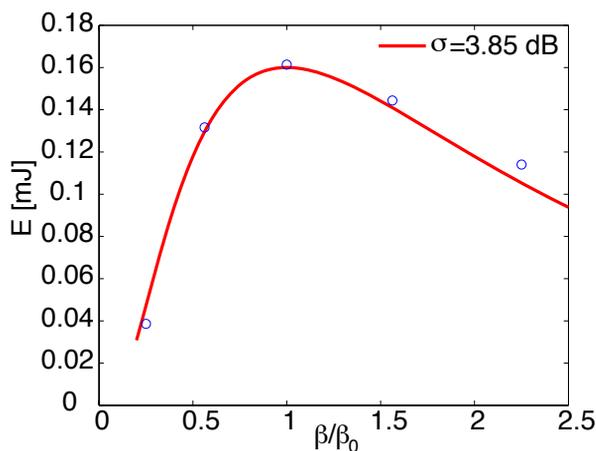
Figure 3: Sensitivity of the FEL energy at the saturation point of the undisturbed FEL performance for the beta-mismatch of the Aramis beam line at one Ångström.
