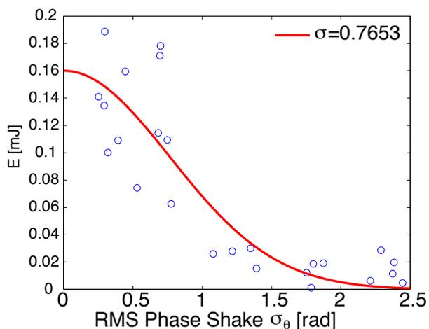
Figure 1: Sensitivity of the FEL energy at the saturation point of the undisturbed FEL performance for the phase shake caused by undulator module detuning of the Aramis beam line at one Ångstrom.
