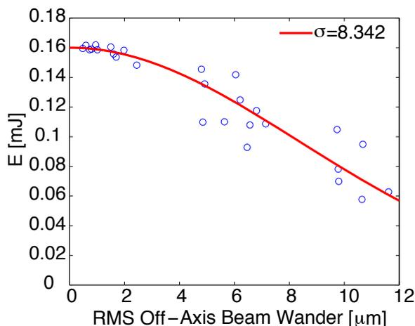
Figure 2: Sensitivity of the FEL energy at the saturation point of the undisturbed FEL performance for the beam wander caused by quadrupole misalignment of the Aramis beam line at one Ångstrom.
