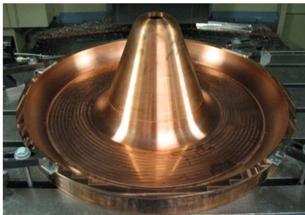
Figure 3: VHF cavity backplane wall with the cathode cone temporarily assembled for mechanical fitting test.
