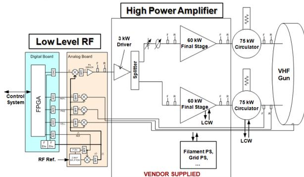
Figure 6: RF power source block diagram.
