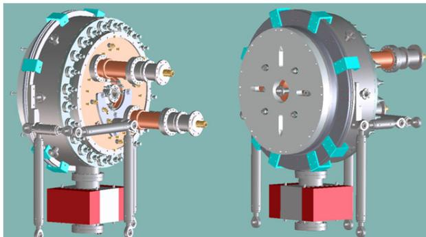
Figure 2: VHF cavity cross-section, showing the cavities main components.
