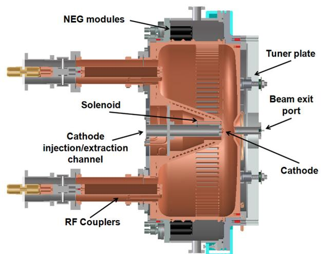
Figure 1: VHF cavity cross-section, showing some of the cavity main components.
