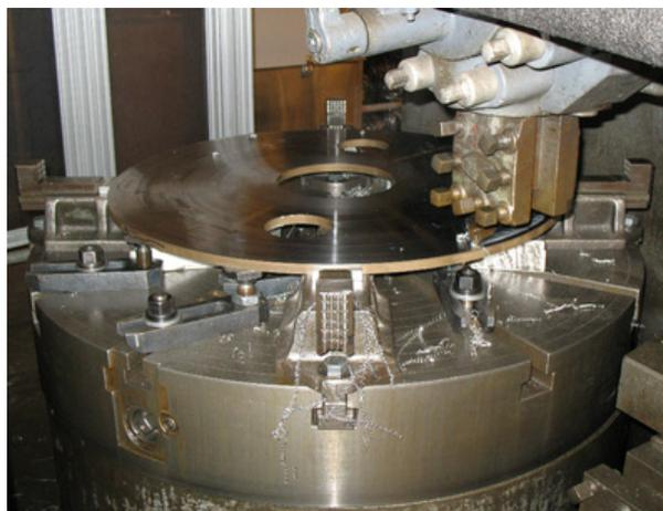
Figure 5: The stainless steel cavity shell backplane wall under machining.
