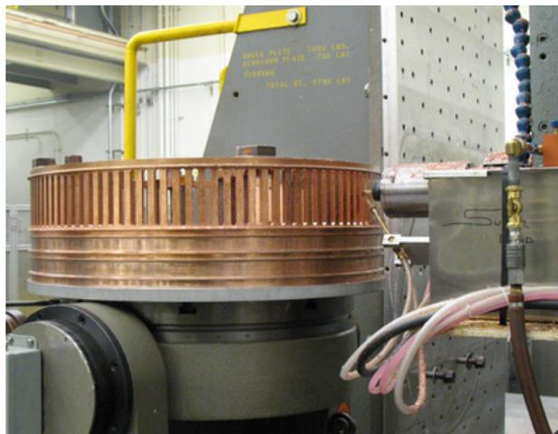
Figure 4: The "coliseum", the side wall of the RF cavity being machined.
