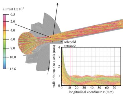
Figure 4: 3D view of electron beam propagation and its projection on the  $r$ - $z$  plane. The colour of the trajectory is a measure of the current it carries.
