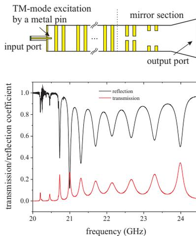
Figure 7: Numerical model of the mirror section and its calculated transmission and reflection coefficient.
