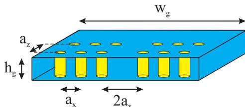
Figure 5: Unit cell of the PHC for the single beam pFEL, consisting of a rectangular waveguide and metal posts of radius  $r = 0.75$  mm,  $a_x = 2.7$  mm,  $a_z = 3$  mm,  $w_g = 18.9$  mm,  $h_g = 8$  mm.
