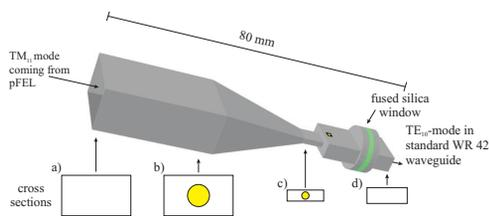
Figure 8: 3D view of the broadband antenna, mode converter and vacuum window
