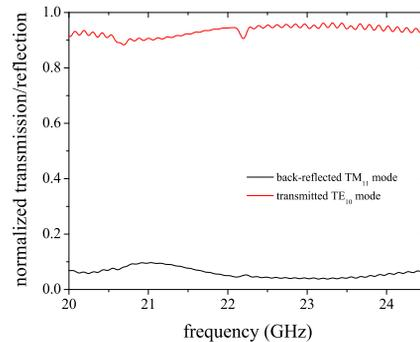
Figure 9: Calculation of transmission and reflection coefficients for the whole device of Fig. 8.
