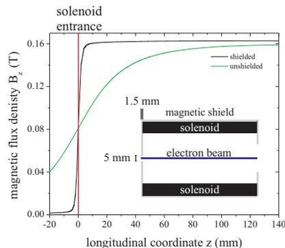
Figure 3: Magnetic flux density produced by the solenoid with (shielded) and with-out (unshielded) end caps. The current density in the solenoid windings is  $6.5 \text{ A/mm}^2$ .
