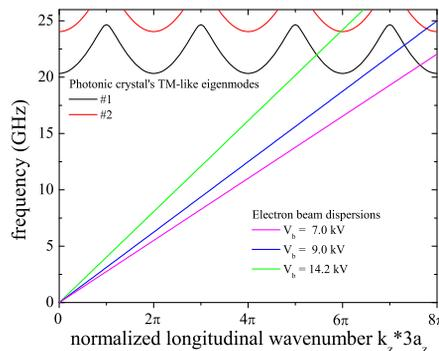
Figure 6: Dispersion of the first two TM-like eigenmodes and electron beam dispersion for several beam voltages.
