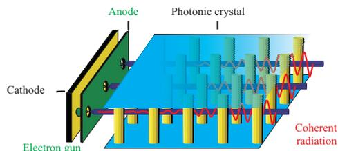
Figure 1: Schematic overview of a pFEL, Not shown: solenoid for electron beam guiding.
