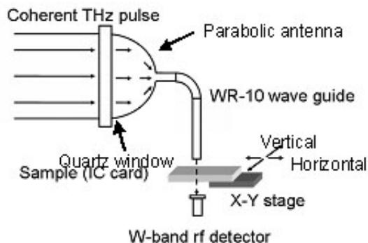
Figure 6: Setup of THz transmission imaging using THz CSR pulse with W-band waveguide, detector and X-Y sample stage.
