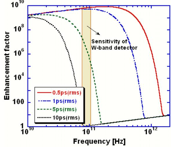
Figure 3: Enhancement factor of CSR as a function of frequency by changing electron rms bunch length (0.5 ps, 1 ps, 5 ps, 10 ps).
