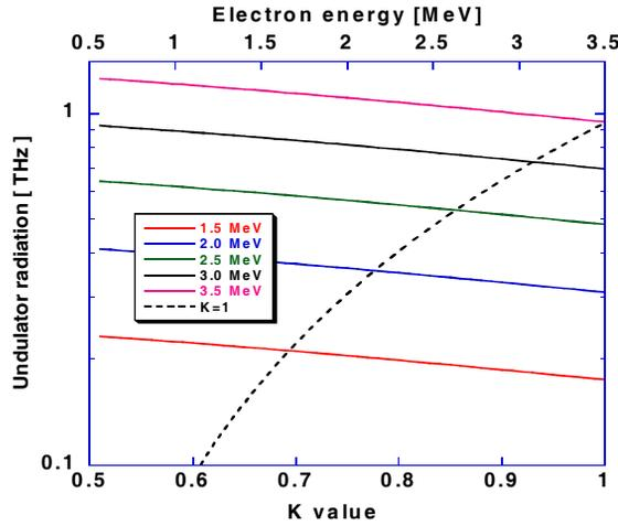
Figure 2: THz Undulator radiation using rf gun.
