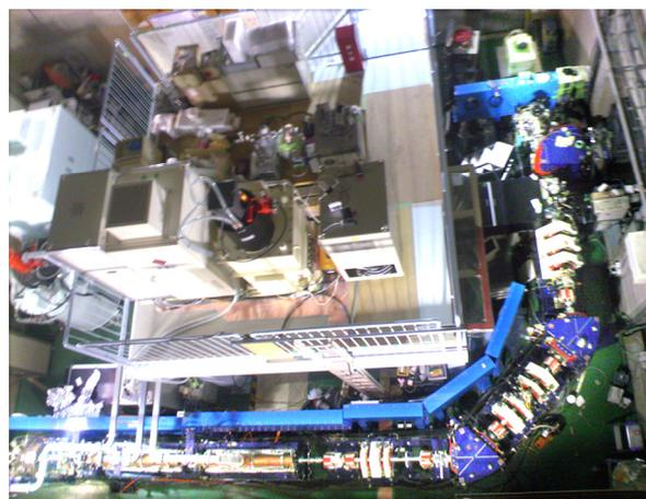
Figure 1: Top view photograph of S-band compact electron linac and mezzanine space for the compact THz FEL based on the photocathode rf gun.
