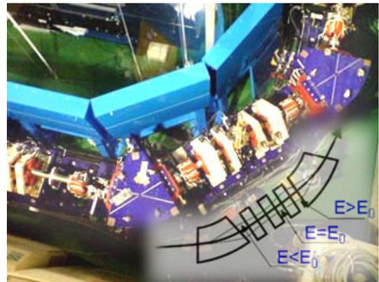
Figure 4: Achromatic arc section for bunch compression.
