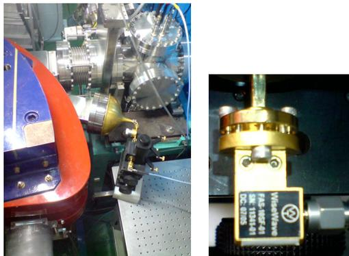
Figure 5: Setup of THz measurement at 90degree bending magnet with W-band rf detector
