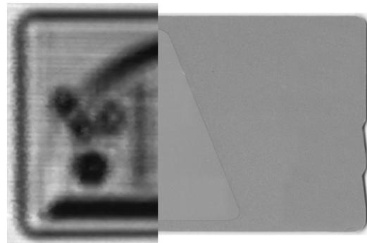
Figure 7: THz transmission image of the left part of IC card with area of  $50 \times 35\text{ mm}^2$ .
