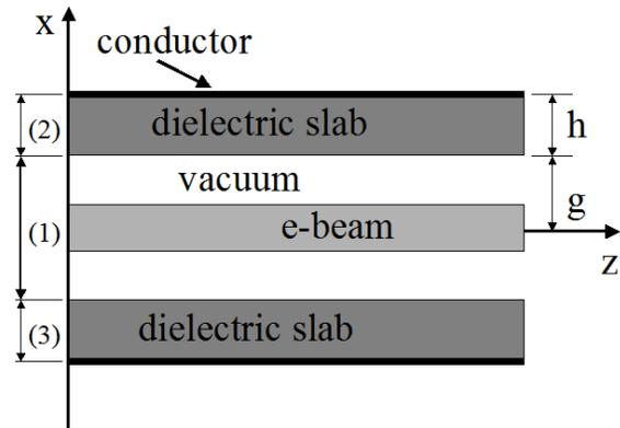
Figure 1: Double-slab Cherenkov free-electron laser
