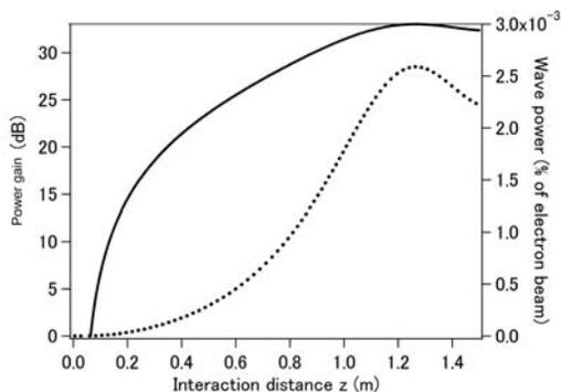
Figure 2: Evolution of power gain (solid line) and radiation power (dotted line) along the interaction region.
