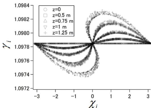
Figure 3: Plots of the energy  $\gamma$  and phase  $\chi$  of the beam electrons for a series of distances along the interaction region.
