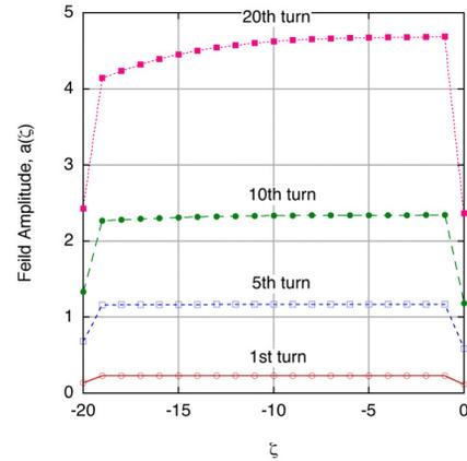
Figure 2: Evolution of the field amplitude at the beginning of lasing. Up to  $\sim 20$  turns, the amplitude grows linearly.
