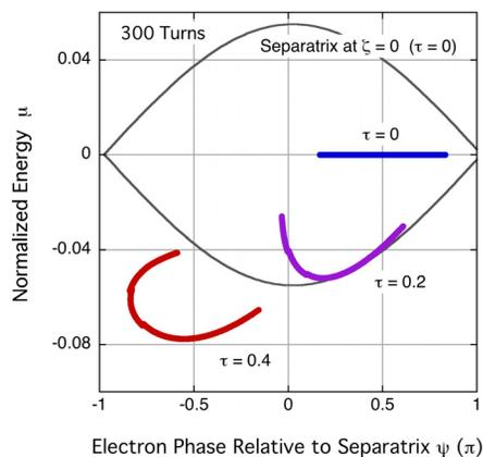
Figure 4: The phase space evolution at 300th round-trip. The bunch phase relative to the 1st slice of optical potential is around  $\pi/2$  at the entrance of the undulator. At  $\tau = 0.4$ , the bunch is passing through the 8th slice because the number of undulator period is 20. As shown in Fig. 3(b), the separatrix of the 8th potential is much smaller so that the bunch is no longer inside of the separatrix.
