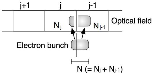
Figure 1: Partition of the electron bunch for calculating the bunching factor in each slice of the optical field.
