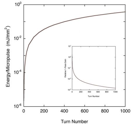
Figure 5: Evolution of micropulse energy plotted as a function of the turn number. Insert shows relative one-pass gain.
