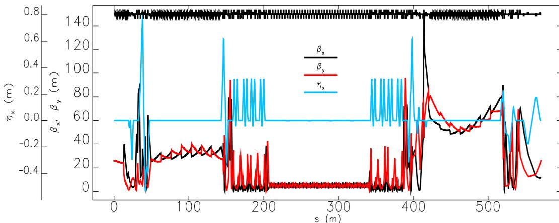
Figure 1: Optics functions from second injector cryomodule to final compressor at the end of the second linac pass.
