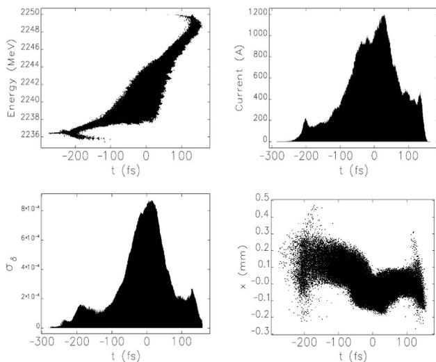
Figure 7: Final bunch properties: (1) longitudinal phase space, (2) current profile, (3) slice energy spread & (4) horizontal-transverse distribution.
