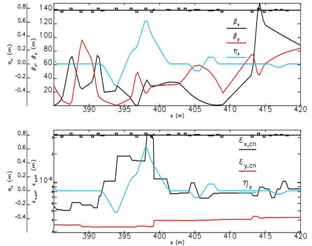
Figure 4: Optics functions and tracked projected normalised emittances at re-injection.
