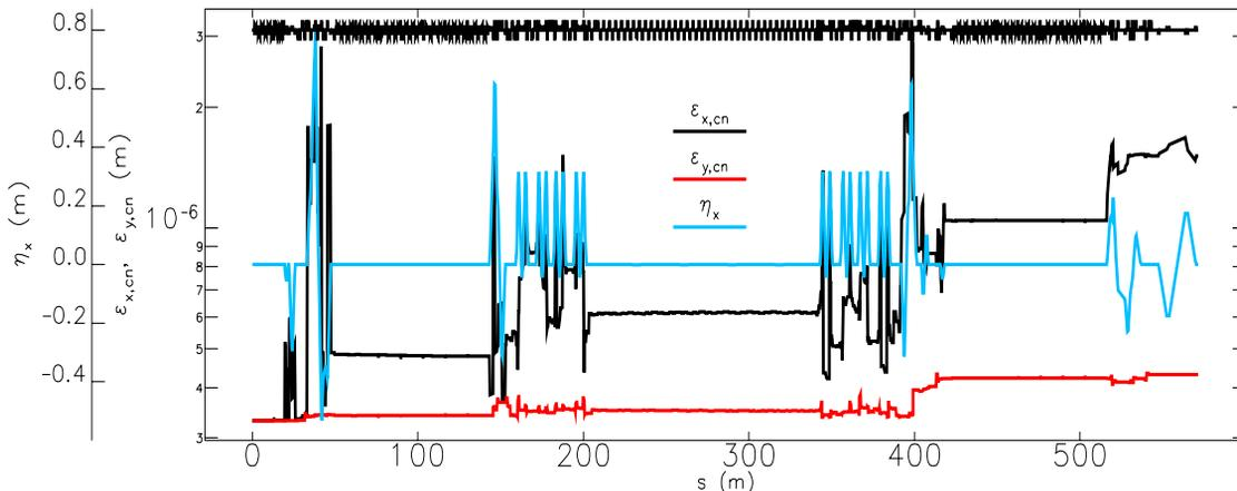
Figure 5: Projected normalised emittances (and horizontal dispersion) through machine.
