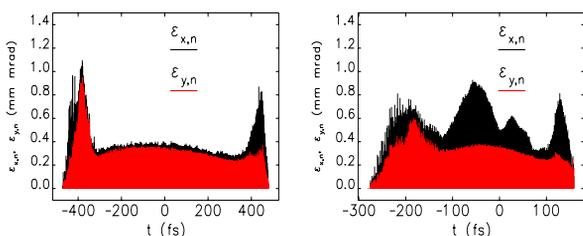
Figure 6: Normalised slice emittances before (left) and after (right) final compression.
