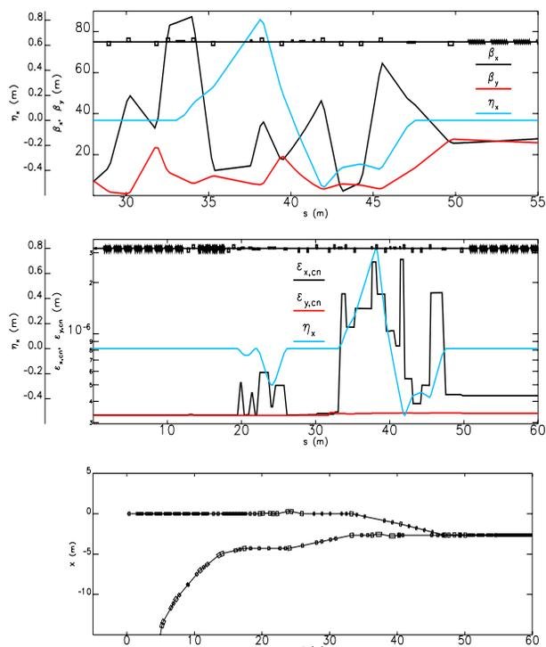
Figure 2: Optics functions, tracked projected normalised emittances and layout of injector.
