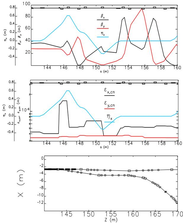
Figure 3: Optics functions, tracked projected normalised emittances and layout of extraction.
