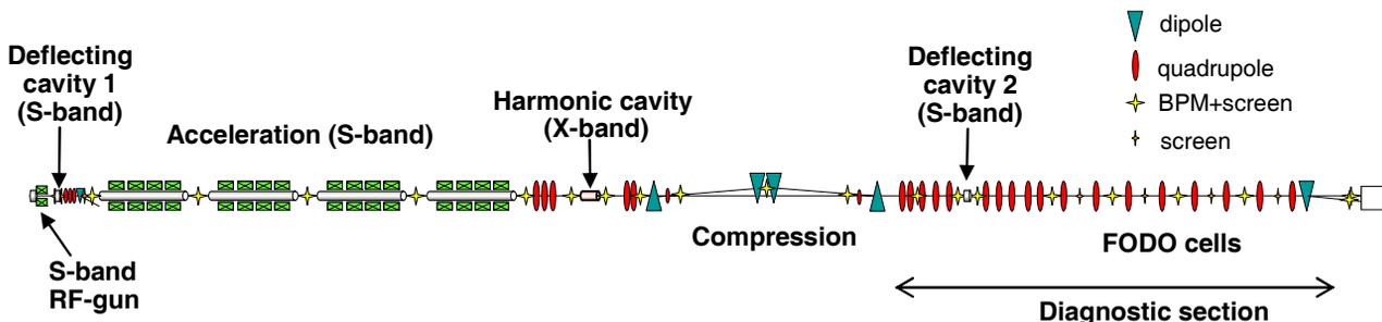
Figure 1: Schematic of the 250 MeV injector test facility.
