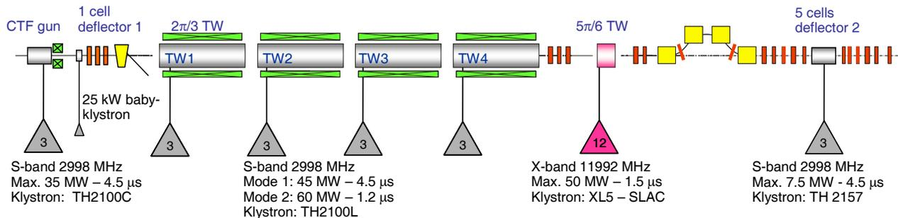
Figure 2: RF systems of the 250 MeV Injector test facility at PSI.
