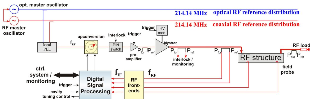
Figure 3: Generic LLRF system for all 3/12 GHz RF stations.
