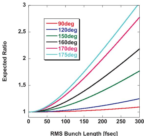
Figure 8: Crossing angle dependence of femto-second bunch measurement.
