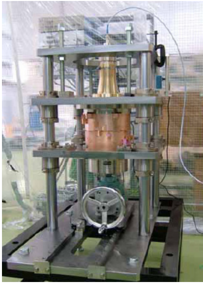
Figure 6: Frequency tuning apparatus of the rf gun cavity.
