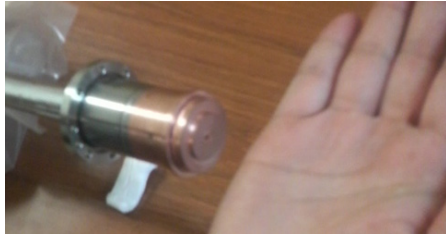
Figure 2: Coaxial cavity to be installed in an existing conventional rf gun.
