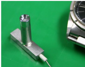
Figure 4: Tungsten cathode of 2-mm diameter with the wehnelt electrode.
