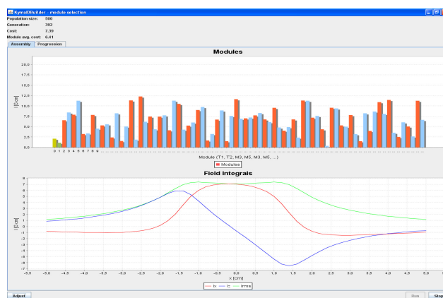
Figure 10: Field integrals computation during the optimization process with Kyma ID Builder.
