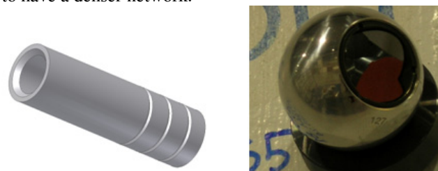
Figure 3: Secondary Socket and CCR placed in a Secondary Socket with a CCR holder
