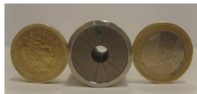
Figure 5: One of the quadrupoles compared with a 1 euro and 1 pound coin.
