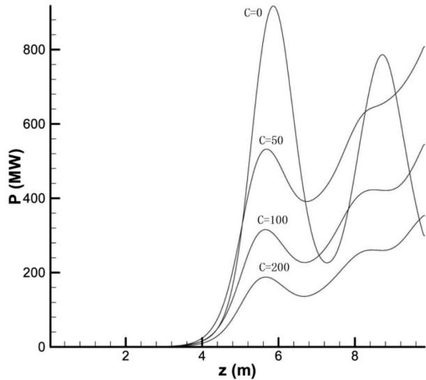
Figure 1: Averaged power of the optical pulse as a function of the undulator length with different initial chirp parameters.
