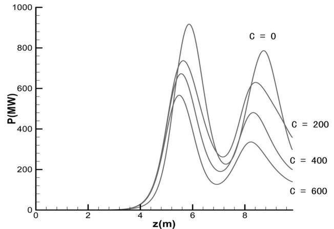
Figure 3: Averaged power of the optical pulse as a function of the undulator length with different initial chirp parameters.
