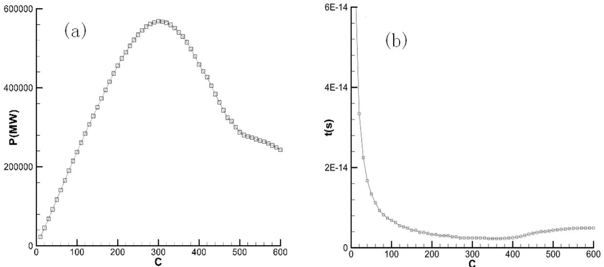
Figure 4: Peak power and FWHM width of the compressed optical pulse vs initial chirp parameter.
