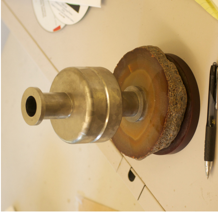
TM_{010} mode superconducting cavity Resonant Frequency 2.865 GHz Q_0 \sim 10^9
