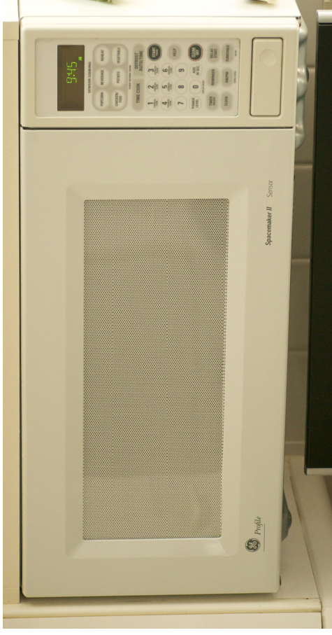
Microwave Oven Multimode Cavity Operating Frequency 2.45 GHz
