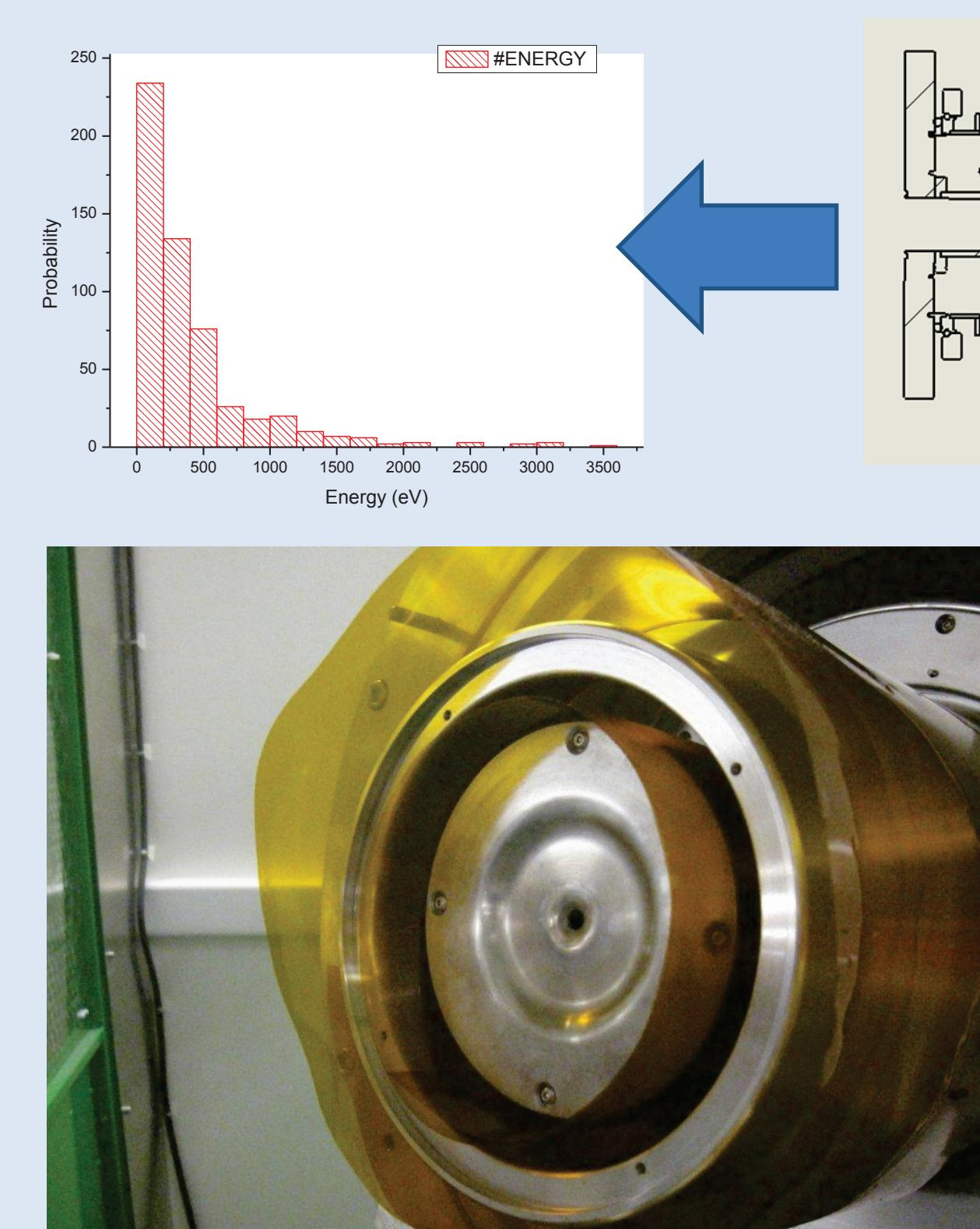
To comfort our idea, we placed around the electrodes several foils of Kapton. We applied simultaneously the HV and the magnetic field several millisecond. We compared the locations of the marks on the foils with the trapped electrons zones simulated with the code: they showed a good agreement.
