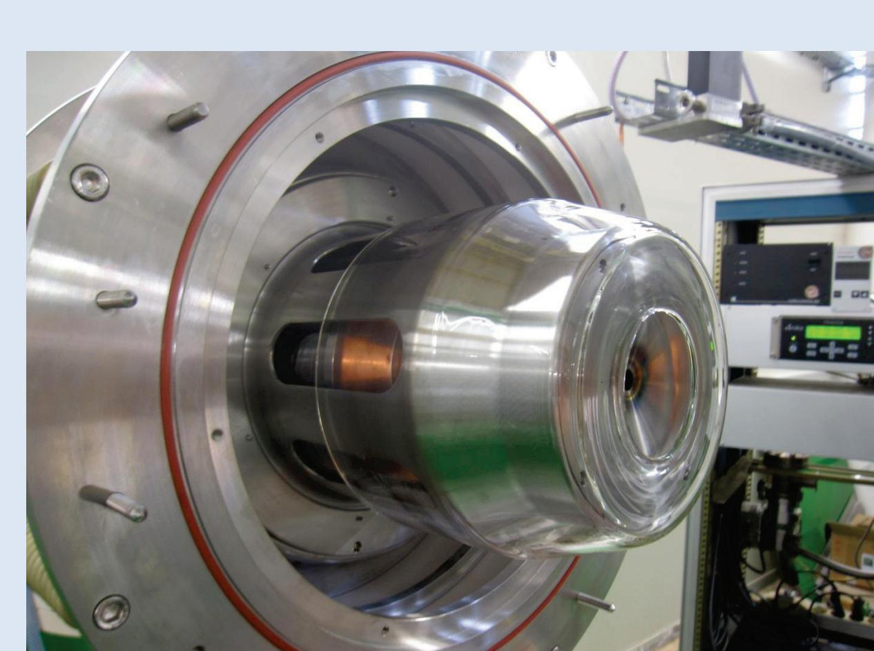
In order to reduce the Penning discharge occurrence, three tubes made of glass were positioned around the electrodes. That allowed us to apply simultaneously HV and magnetic field in order to ignite the ECR plasma and extract the H<sup>+</sup> particles out of the source.
