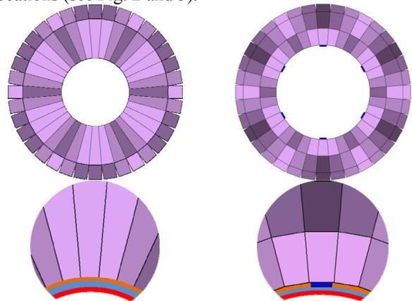
Figure 4: Up: Hexapole cross section of PHOENIX V2 (left) and V3 (right). Down: zoom on plasma chamber detail for V2 (left) and V3 (right).
