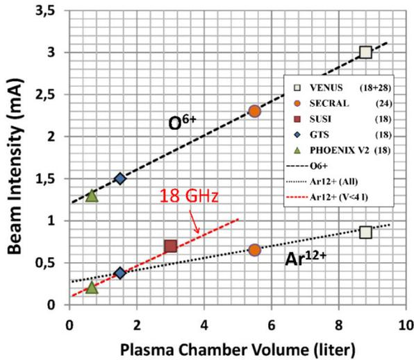
Figure 3: A/Q=3 beam current evolution for various ECRIS as a function of the chamber volume.
