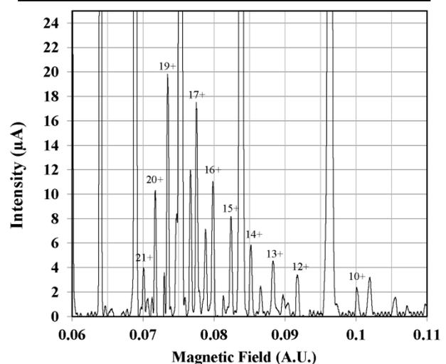
Figure 1: Nickel spectrum obtained with PHOENIX V2.
