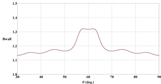
Figure 7: Magnetic boost along the wall induced by one of the iron plates, as a function of the azimuthal angle ( $\theta=60^\circ$  is a main pole, next pole would be  $\theta=120^\circ$ ,  $r=45$  mm,  $Z=0$  mm (centre of the source)).
