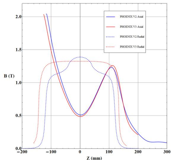
Figure 5: Axial (solid line) and radial (dashed line) magnetic field intensity along the source axis. Wall generated by the sole hexapole (dashed). Red and blue curves stand respectively for PHOENIX V3 and V2.
