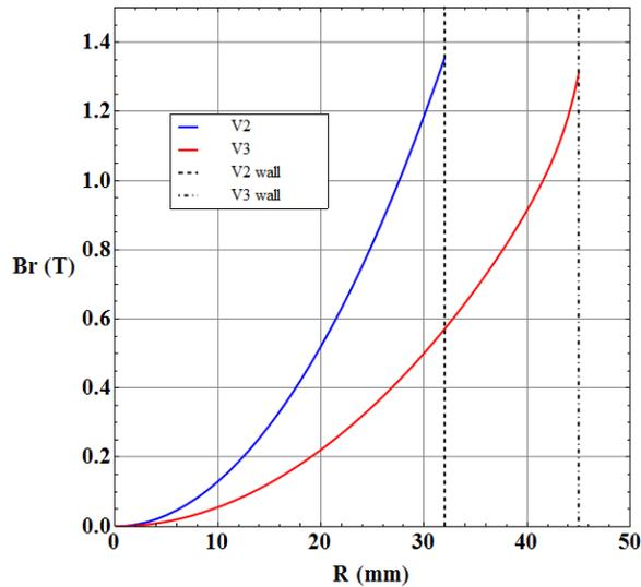
Figure 6: radial magnetic intensity in the center of the source generated by the hexapole as a function of the radius for PHOENIX V2 (blue) and V3 (red). Dashed lines stand for plasma wall position.
