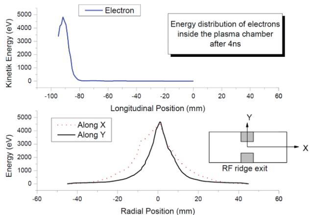
Figure 5: Spatial-energy distribution of electrons in the plasma chamber calculated with SOLMAXP.
