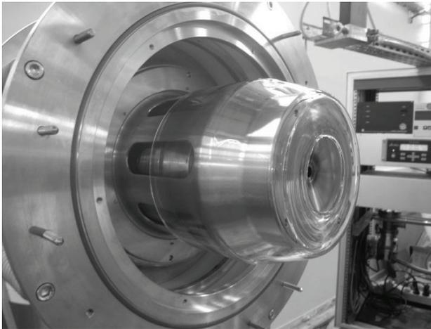
Figure 3: External glass-tube around the puller electrode.
