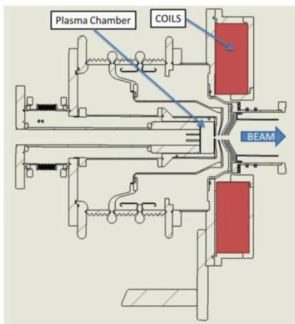
Figure 1: ALISES Ion Source, extraction side.
