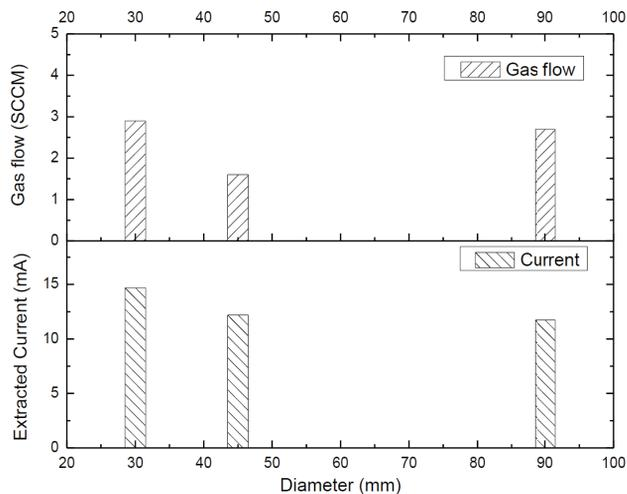
Figure 6: Extracted current intensity and injected gas pressure versus plasma chamber diameter.
