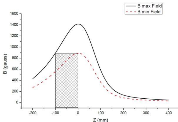
Figure 2: Fringe field of the source coil. The dash zone represents the plasma chamber
