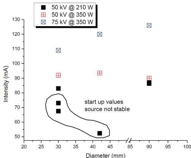
Figure 7: Preliminary results on IFMIF source, intensity vs plasma chamber diameter, bias voltage and beam extraction energy.
