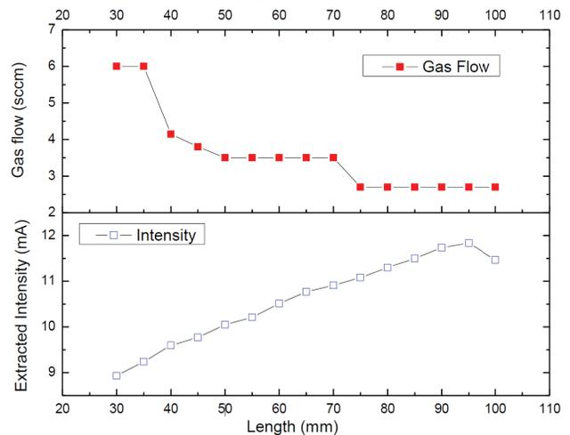
Figure 4: Intensity extracted and injected H<sub>2</sub> gas flow versus plasma chamber length.
