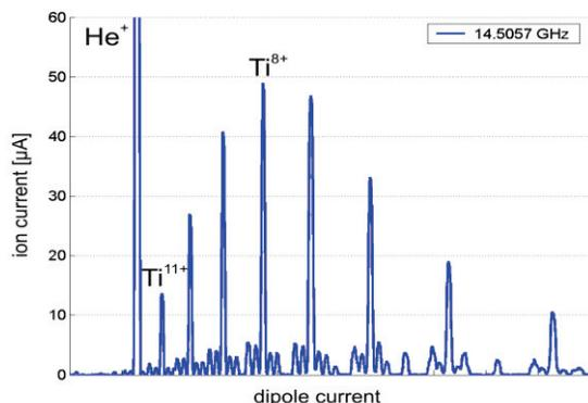
Figure 6: Mass/charge spectrum of natural Ti (forward power = 250 W; reflected power = 28 W; HTO heating power = 234 W).
