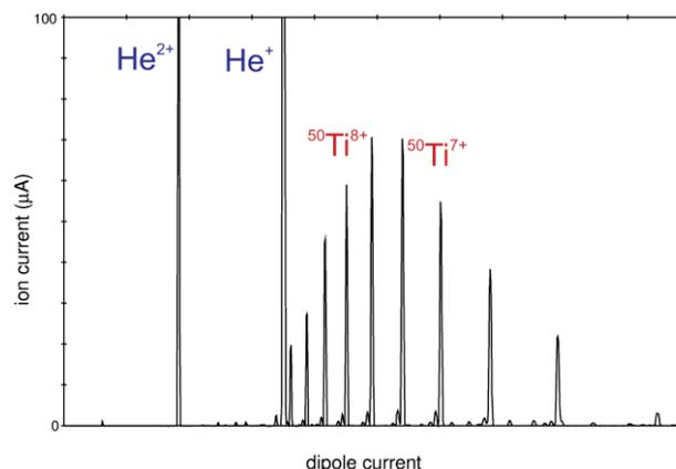
Figure 5: Typical mass/charge spectrum of  $^{50}\text{Ti}$ .
