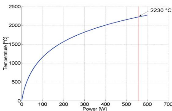
Figure 4: HTO temperature as function of heating power (measured up to 2050°C; extrapolated above 2050°C).
