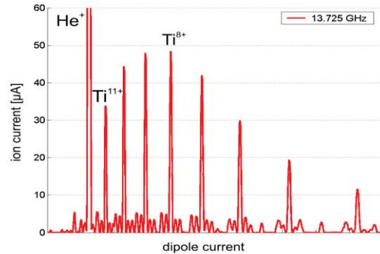
Figure 7: Mass/charge spectrum of natural Ti (forward power = 250 W; reflected power = 1 W; HTO heating power = 234 W).
