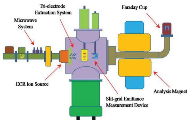
Figure 1: The skeleton diagram of PKU Ion Source Test Bench.
