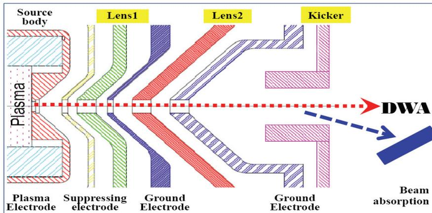
Figure 3: The schematic view of AISLI (un-scaled).
