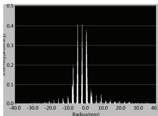
Figure 2: The transverse distribution of 50 mA/40 keV H<sup>+</sup> beam at the location of DWA entrance.
