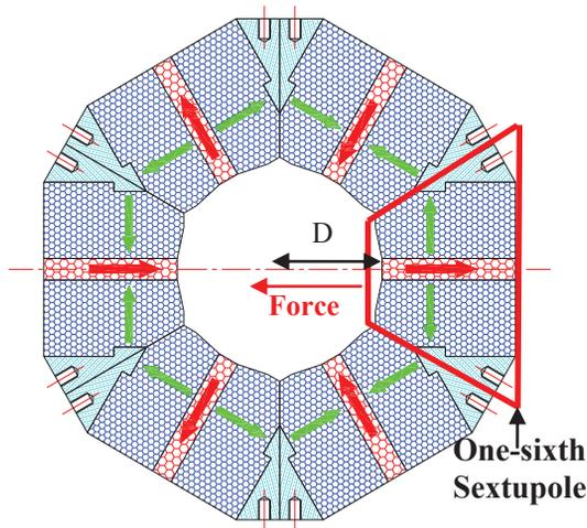
Figure 4: The layout of LECR4-DRAGON ECR ion source sextupole magnet and force analysis of one-sixth sextupole magnet.
