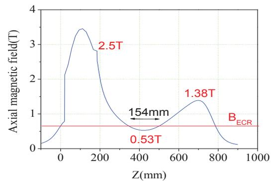
Figure 2: The axial field profile of DRAGON that is similar to the SECRAI operation at 18 GHz. With an iron plug field booster the maximum axial field reaches 2.5 T at the surface of the bias probe in the injection.
