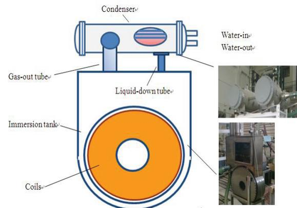
Figure 3: Schematic layout of evaporative cooling system for LECR4-DRAGON.
