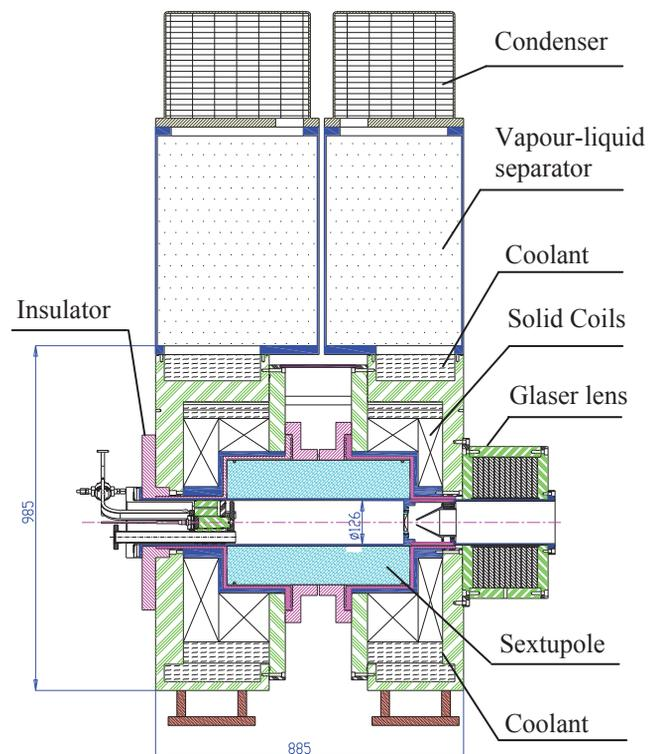
Figure 1: A schematic cross-section view of the LECR4-DRAGON. No mechanical pumping at the injection side for simplicity but may be added in the future.
