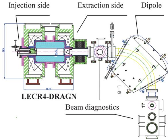
Figure 5: Layout of LECR4-DRAGON ECR ion source and its beam transport line.
