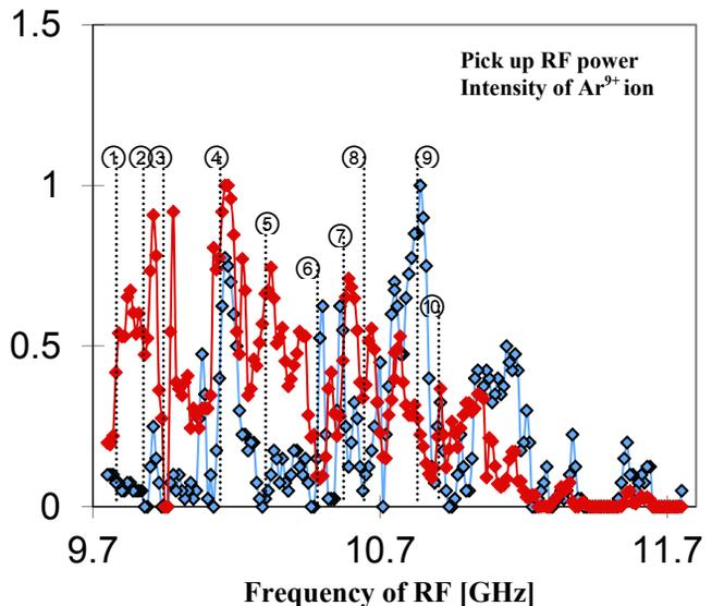
Figure 4: Measured Beam intensity of  $\text{Ar}^{9+}$  and Pick up voltage strength of plasma chamber vs RF frequency.
