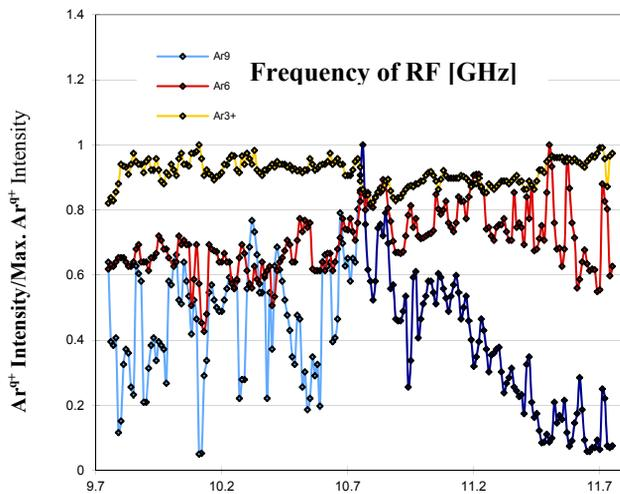
Figure 2:  $\text{Ar}^{9+}$  Intensity vs RF frequency ( $\text{Ar}^{9+}$  intensity (normalized by maximum current, respectively) vs RF frequency).
