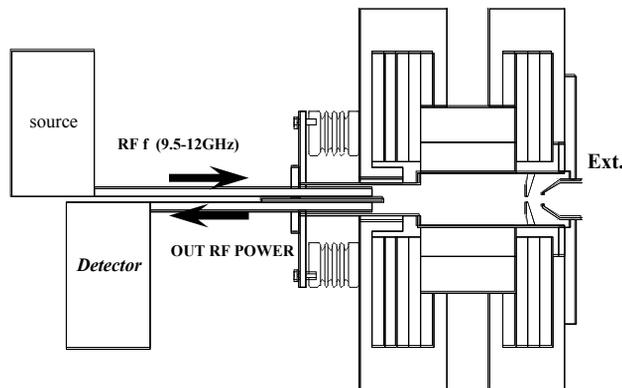
Figure 1: Experimental Apparatus and FM-ECR ion source.
