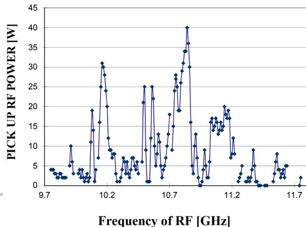
Figure 3: Measured pick up voltage strength of plasma chamber vs RF frequency.
