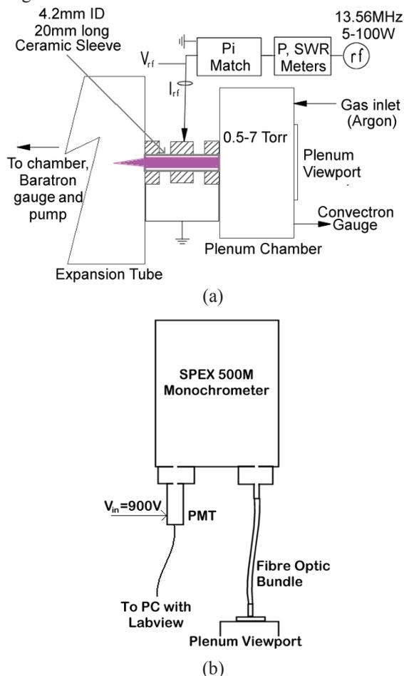
Figure 1: Experiment setup (a) Pocket Rocket System and (b) Spectroscopy equipment setup
