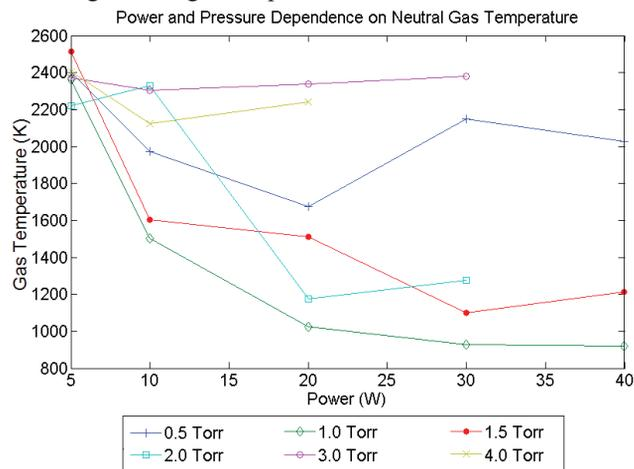
Figure 4: Neutral gas temperatures for an argon nitrogen plasma discharge for input powers of 5-40W and upstream pressures of 0.5-4.0Torr.
