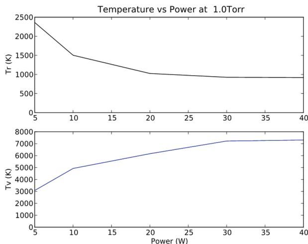
Figure 5: Change in rotational and vibrational temperature with power for a 1.0 Torr argon-nitrogen plasma.
