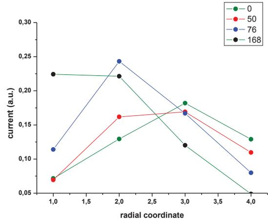
Figure 5: Dependence of the plasma flux radial profile on the value of the biased potential for the value of the magnetic field at the plug of 1.3 T.
