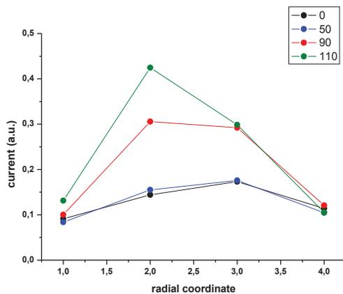
Figure 4: Dependence of the plasma flux radial profile on the value of the biased potential for the value of the magnetic field at the plug of 1.5 T. For this case the shift of the profile maximum observed at the value of the voltage close to the 90 V.
