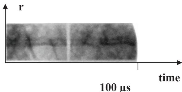
Figure 7: Streak camera image for the limiter potential of 120 V.
