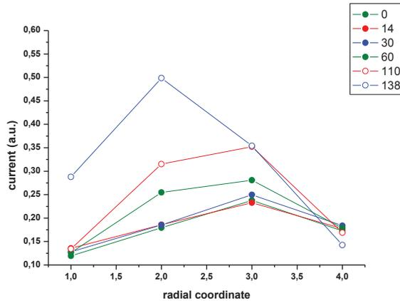
Figure 3: Dependence of the plasma flux radial profile on the value of the biased potential for the value of the magnetic field at the plug of 1.7 T. Radial coordinate 1 corresponds to the 1<sup>st</sup> probe, 2 – for second, etc.
