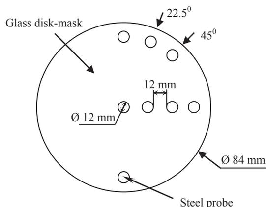
Figure 2: Scheme of the probes positioning in the probe's system.
