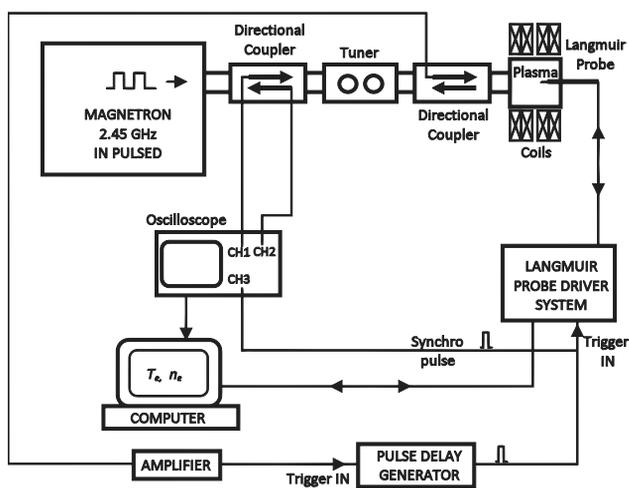
Figure 2: Experimental arrangement for time resolved density and temperature measurements during breakdown with a resolution of 200 ns.
