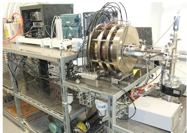
Figure 1: View of the experiment where the plasma reactor, magnetic coils and diagnostic port are shown in first plane.
