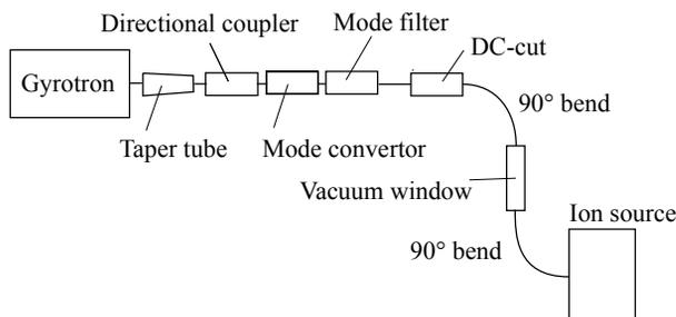
Figure 4: Microwave transmission line.
