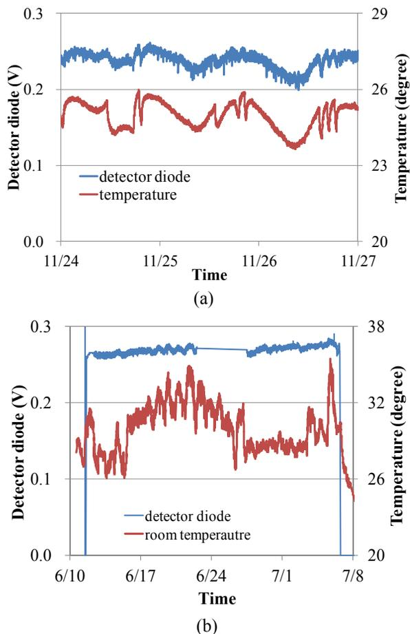
Figure 7: Detector diode voltage for the RF power and the room temperature during operation as a function of time (a) before and (b) after the stabilization of the output RF power.
