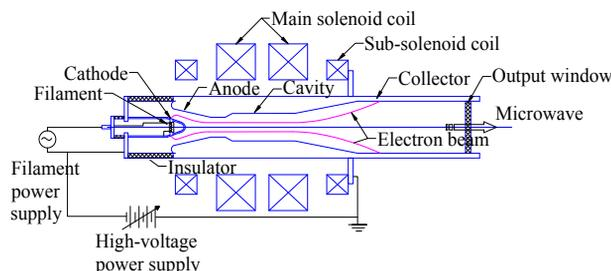
Figure 1: Schematic drawing of the 28 GHz gyrotron.
