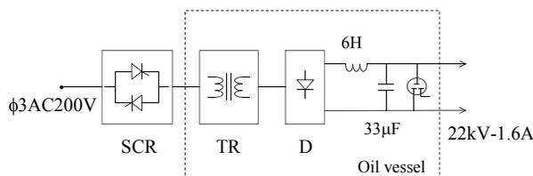
Figure 2: Electric circuit of the cathode power supply.
