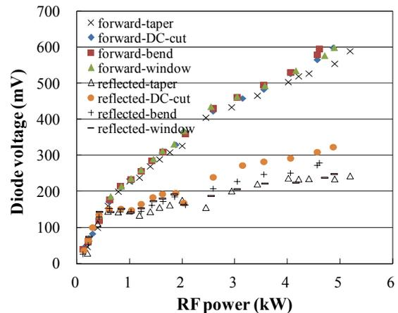
Figure 5: Output of the diode detector.
