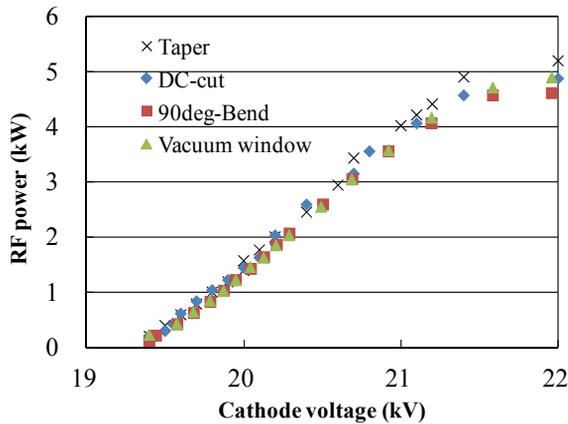
Figure 3: RF power versus cathode voltage.
