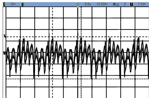
Figure 6: Waveform from the diode detector before improvement. Scales are 10 ms/div and 5 mV/div.
