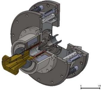
Figure 9: Schematic view of C-ADS proton source.
