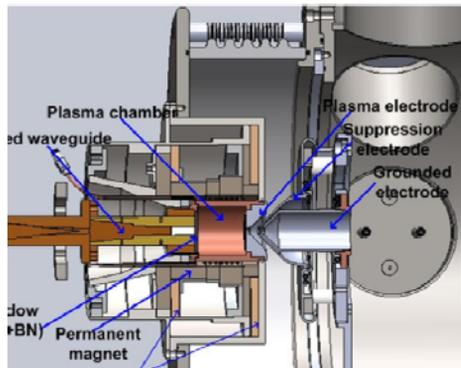
Figure 3: CPHS proton source with 3-electrode extraction.
