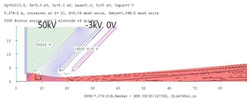
Figure 5a: Simulation result of 3-electrode extraction.
