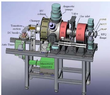
Figure 2: Layout of the proton source and LEBT.
