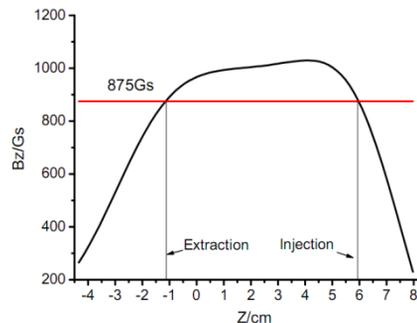
Figure 4: Simulated magnetic field of SPHS Proton Source.
