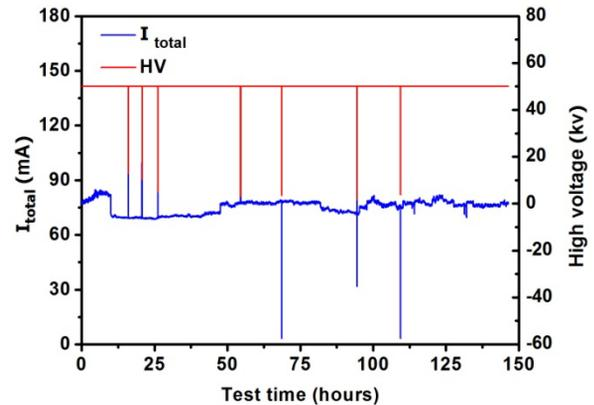
Figure 8: Long time running test of the proton source.
