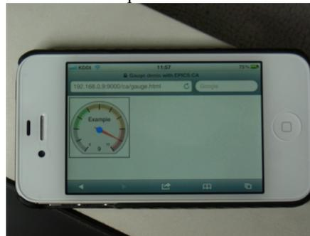
Figure 5: WebSocket-based Web application displayed on iPhone4S.
