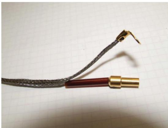
Figure 2: Modified electrical connection for the intermediate electrode.
