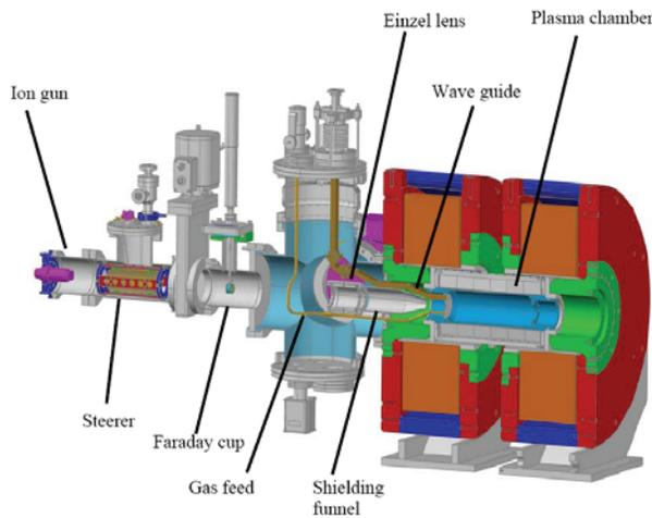
Figure 2: Injection Line into the CB-ECRIS.
