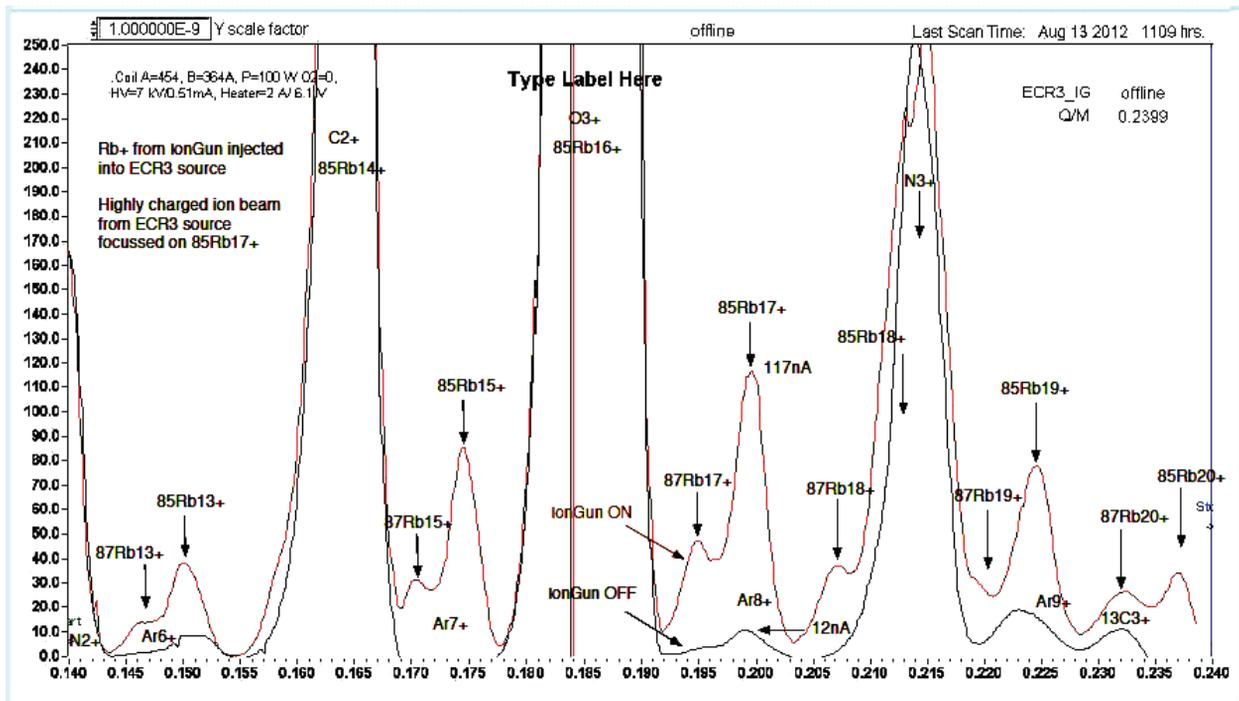
Figure 4: Superimposed spectra with the rubidium beam injected and not injected. The lower scale is charge-to-mass ratio, and the left-hand scale is intensity in nanoamperes.
