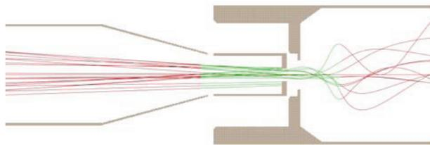
Figure 3: SIMION calculation of injection.
