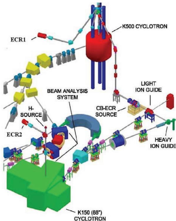
Figure 1: Layout of the Texas A&M Radioactive Beam Facility.
