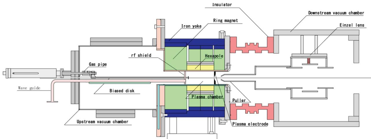
Figure 1: Schematic drawing of Kei3 source.
