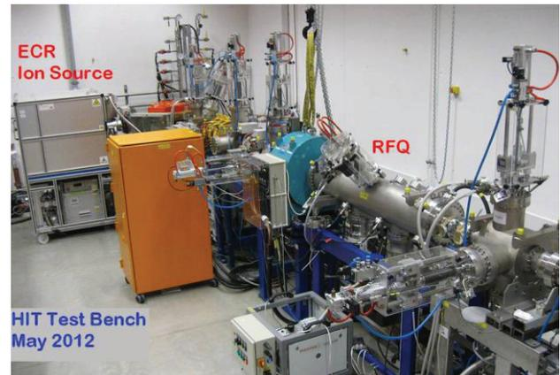
Figure 11: Test bench set up to analyse the RFQ output parameter.
