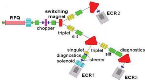
Figure 9: Considered design of the LEBT including three ion sources (planned in winter 2012) (Setup 2).
