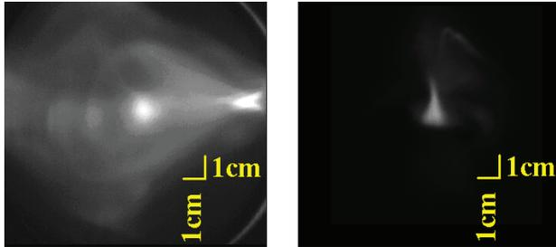
Figure 8: Shape of  $H_3^+$  beam at a glass viewing screen (Herasil) behind the switching magnet. Left figure: Before LEBT modification (2mA) - Right figure: Status now (700e $\mu$ A).
