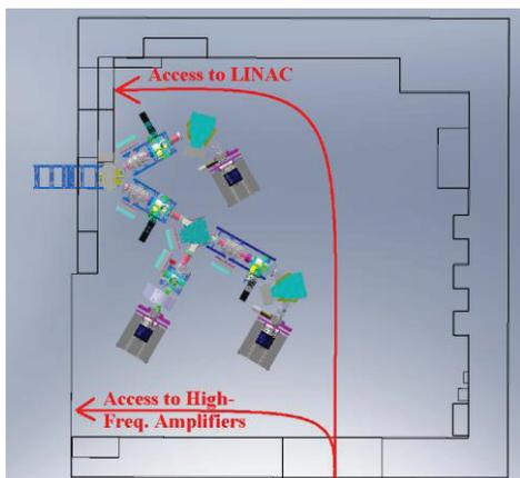
Figure 10: Considered design of the LEBT including three ion sources in the LEBT room.
