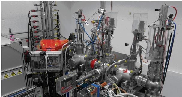
Figure 4: Test bench setup with a slit grid emittance measurement device.
