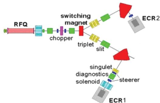
Figure 5: Schematic drawing of the LEBT after winter 2011.
