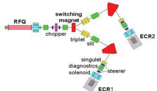
Figure 3: Schematic drawing of the LEBT before winter 2011.
