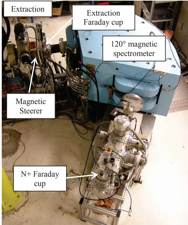
Figure 1: The LPSC charge breeder extraction beam line.
