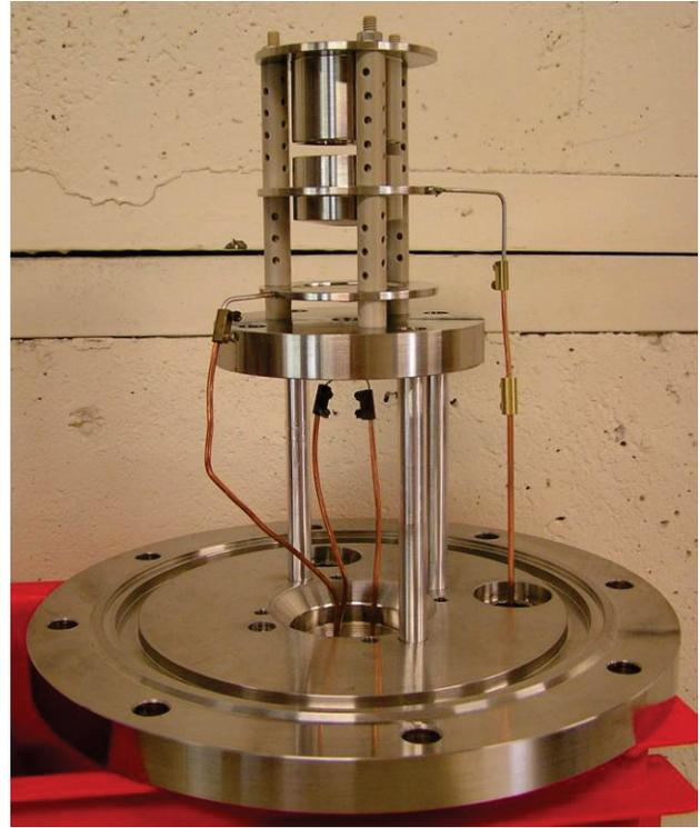
Figure 6: ion gun with its set of three electrodes.
