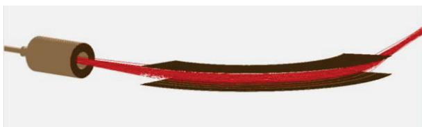
Figure 3: Ion beam trajectories in the magnetic spectrometer after the extraction.
