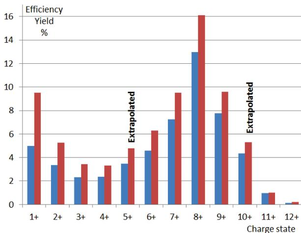
Figure 5: Argon charge state distribution extracted from the LPSC charge breeder.
