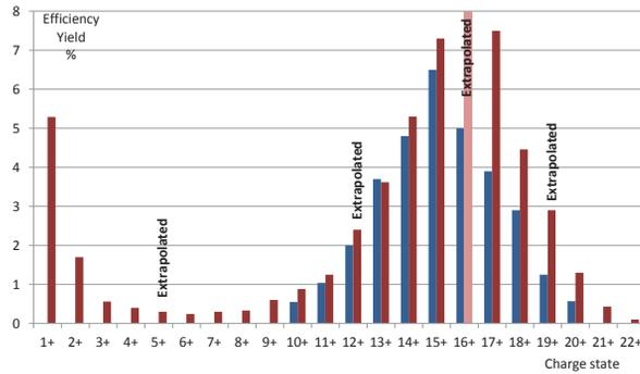
Figure 7: Rubidium charge state distribution extracted from the LPSC charge breeder.
