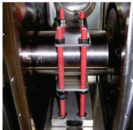
Figure 4: High voltage cylindrical electrode.
