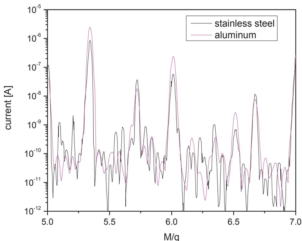
Figure 2: Ion current as function of  $M/q$  ratio for a stainless steel and aluminium plasma chamber.
