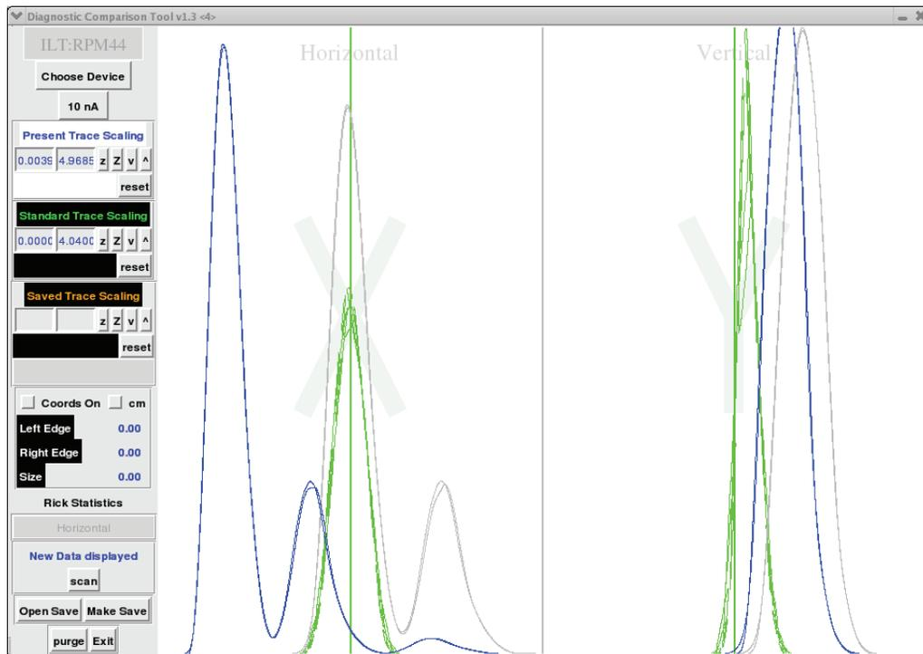
Figure 1: Cs<sup>23+</sup> beam profile (blue) at the focal plane of first bender in front of the RFQ. The center of the beam has been moved in horizontal (x) direction to show more beam components.
