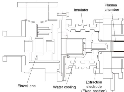
Figure 4: Schematic view of the extraction system of KeiGM.
