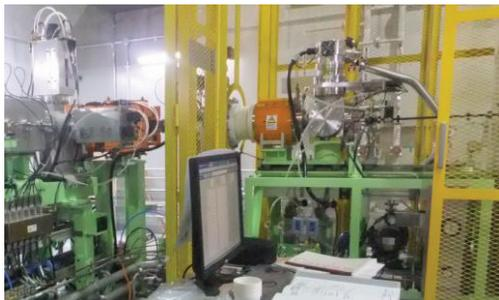
Figure 5: ECR ion source has been installed in SAGA-HIMAT just before launch.
