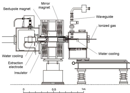
Figure 2: Schematic view of NIRS-ECR ion source.
