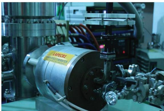
Figure 1: LAPECR1 source installed on a HIRFL injection beam line.
