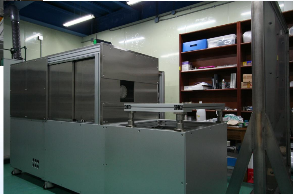
After X-ray shielding (20mm lead)
