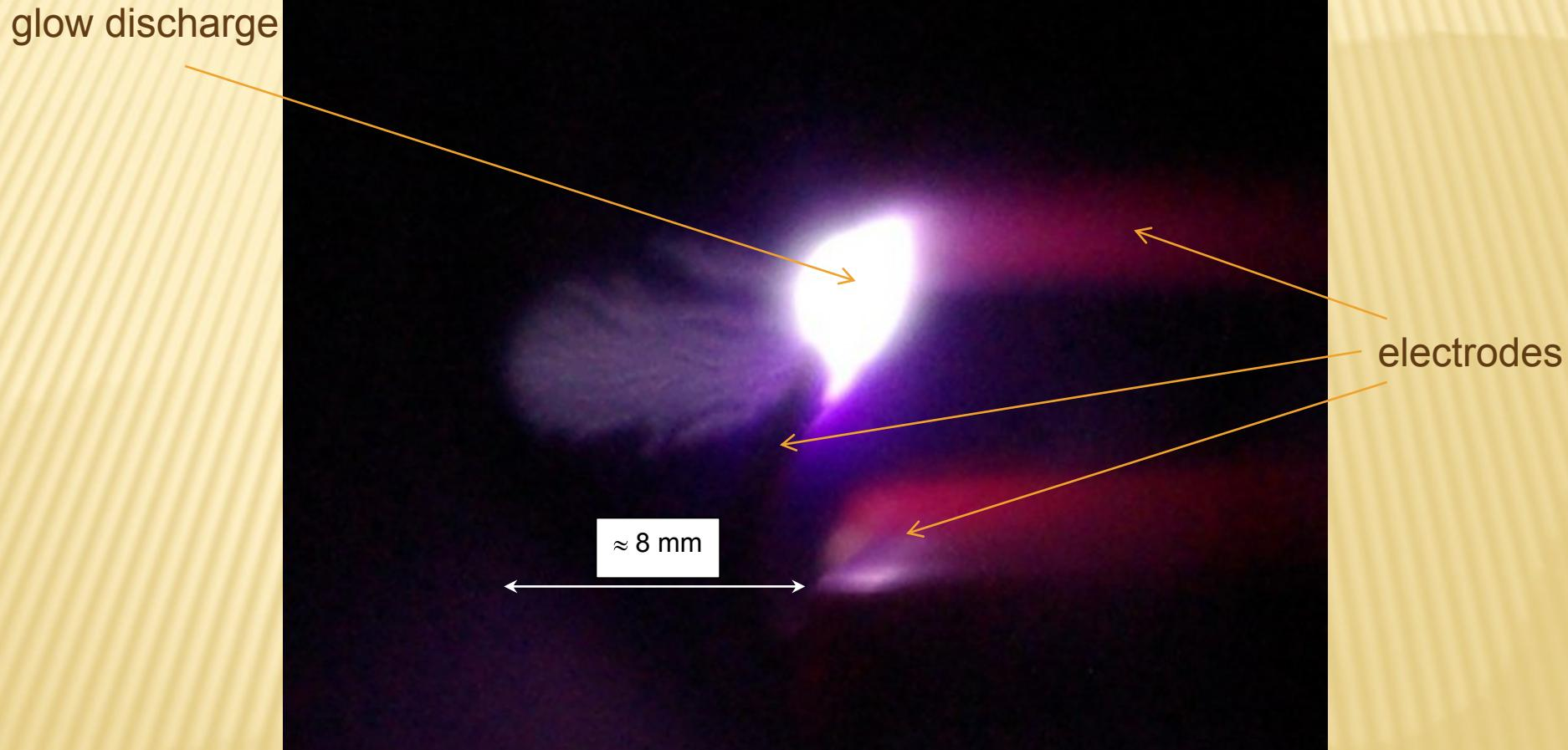
Velocity of discharge propagation more than  $10^5 \text{ cm/s}$
