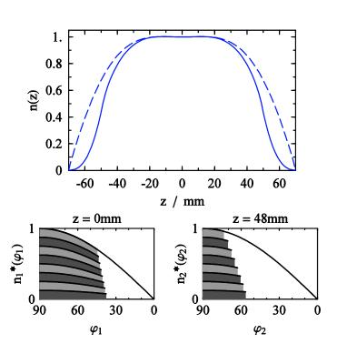
The ratio of cold to hot electrons is strongly related to the electron density ratio in the middle and at the edge of the ECRIS
