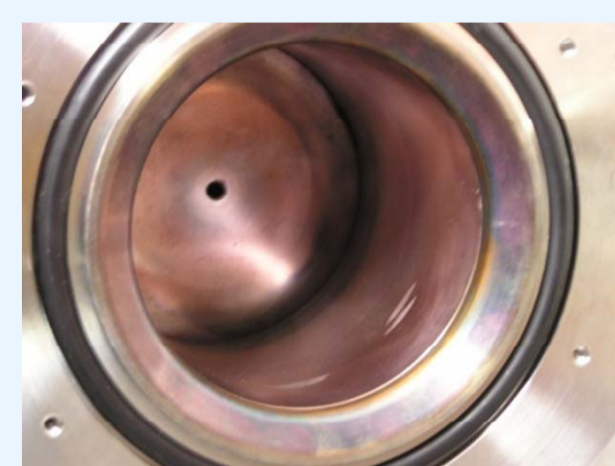
Plasma electrode after test Melted Faraday cup after 20mA measurements
