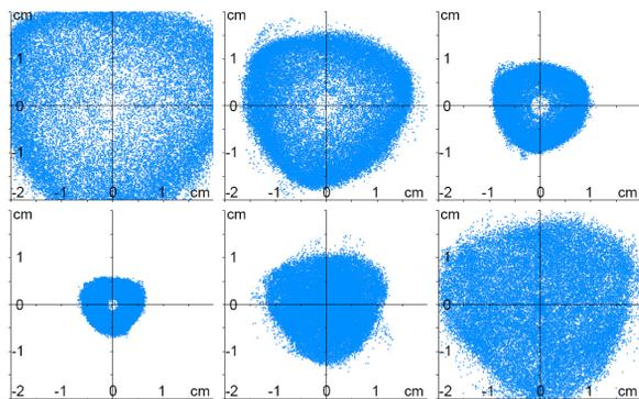
Figure 6: Influence of increasing focal strength of the solenoid on the ion beam profile. The beam is hollow if under focused (first line, focusing force 76%, 83%, and 90%), and becomes triangular afterwards (second line, focusing force 96%, 103%, and 110%).
