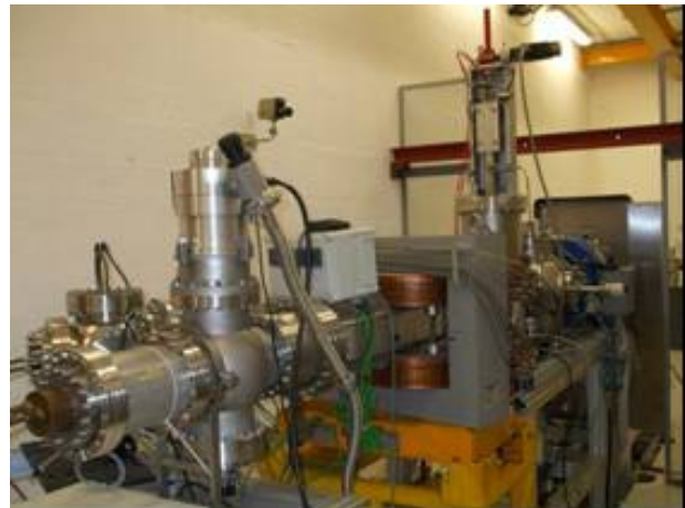
Figure 1: The VIS Source with the Emittance Measurement unit.
