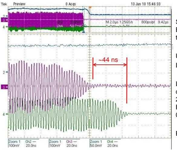
Signals from toroid and two BPM buttons, all downstream of the RFQ
