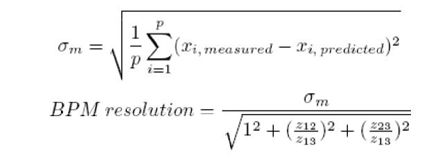
The resolution is nearly 4  $\mu$ m, with a bunch charge of 50 pC up to 270 pC, value that has to be improved with many changes in the electronic system, that are:
