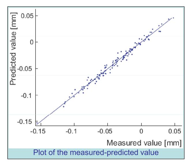
This resolution method compares the reading of the electron beam offset measured with the BPM of interest ('m'), with the predicted value by all the other BPMs [3]. The data is acquired in real time mode, in presence of beam jitter.
