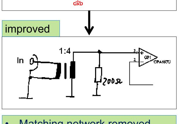
Matching network removedTransformer added
