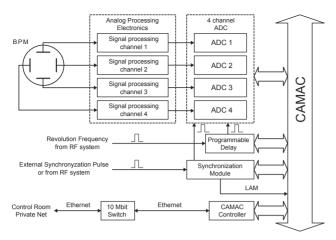
Figure 2: Structure of VEPP-2000 electronics.
