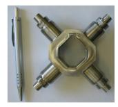
Figure 1: The beam position monitor for VEPP-2000 ring.
