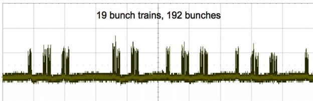
Figure 9: Zoom factor 10^2 (10 \mu s/div): The bunch-train structure shows 8x16 and 3x8 bunch trains, corresponding to 152 bunches in total.
